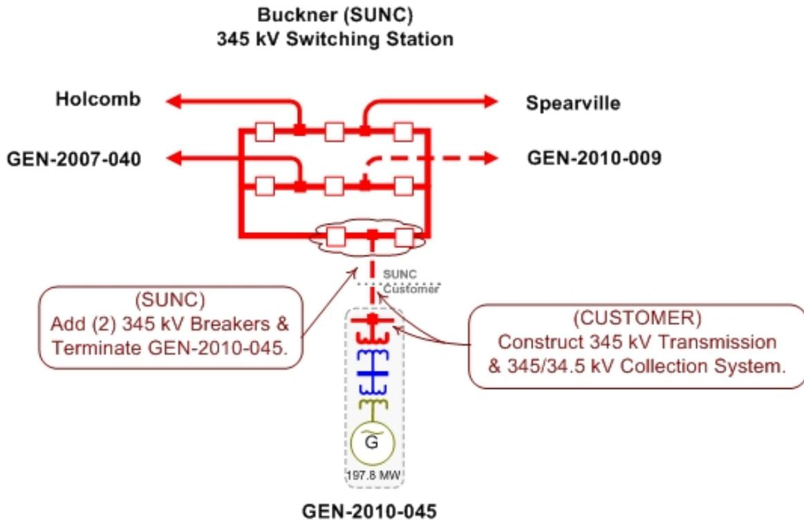
**2.1. Customer Facilities** – The Customer will be responsible for its Generating Facility and its 345/34.5 kV substation that will contain its 345/34.5 kV transformer(s) and wind turbine collector feeders. In addition, the Customer will be required to install the following equipment in its facilities.
